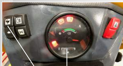
Super bright LCD Display IP67 rated
