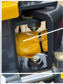
Protected hose lines
