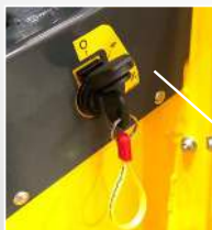
Two stage start inhibitor safety system
