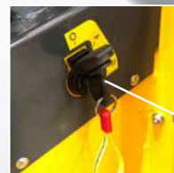
Two stage start inhibitor safety system
