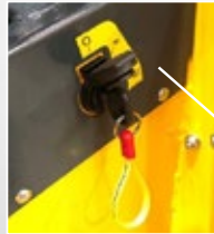
Two stage start inhibitor safety system
