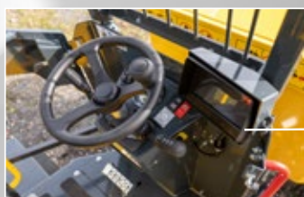
Protected IP67 rated 7" LCD Monitor
