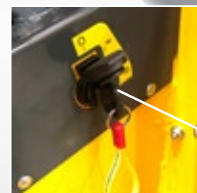
Two stage start inhibitor safety system
